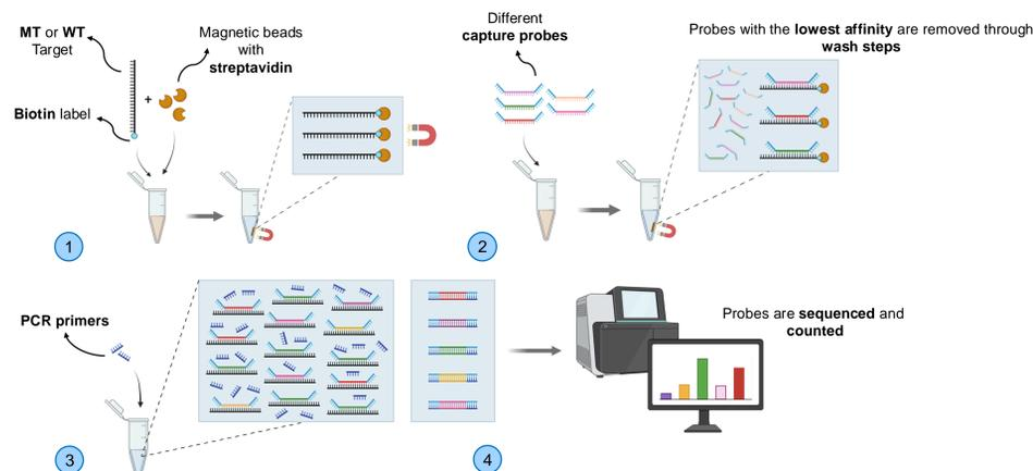
**Fig. 2:** 1) Hundreds of candidate bio-recognition elements (capture probes) that are flanked by PCR handles are hybridized to a biotinylated MT or WT target. 2) Following streptavidin pull-down, 3) probes are converted into a probe library 4) which is quantified by next generation sequencing (NGS).
